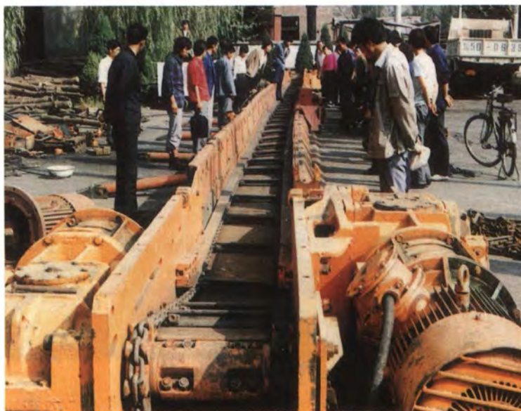
▷象山煤矿创煤机地面试运转
